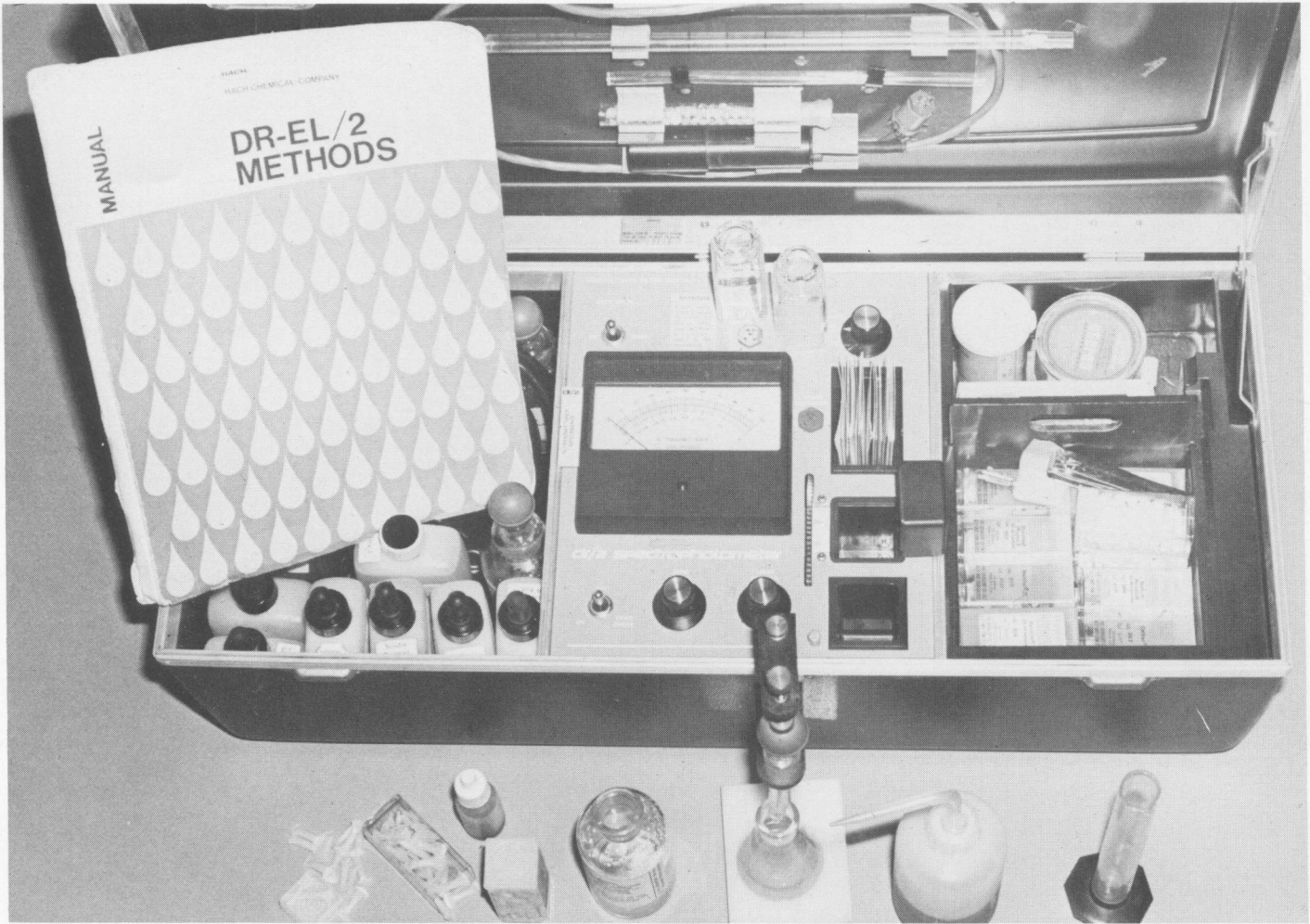
FIG. 27. A large water analysis kit used in fisheries management and occasionally in fisheries research.
