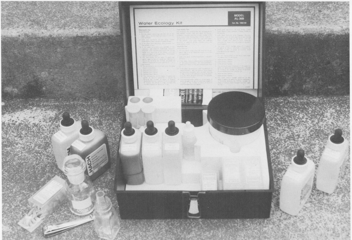
FIG. 23. A small water analysis kit suitable for use in fisheries management.
