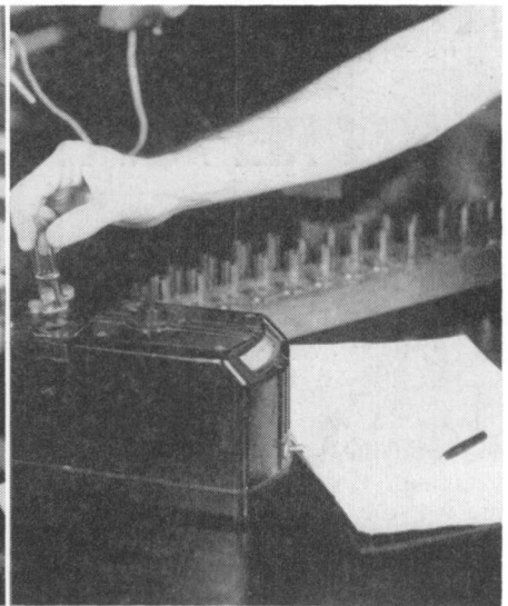
6 The amount of available phosphorus present in the soil is measured with a colorimeter.
