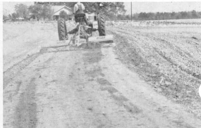
FIG. 1. Power-driven rotary cutters leave the stalks in shreds. FIG. 2. Smoothing a terrace with a land leveler before planting.
