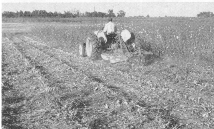
FIG. 1. Power-driven rotary cutters leave the stalks in shreds. FIG. 2. Smoothing a terrace with a land leveler before planting.
