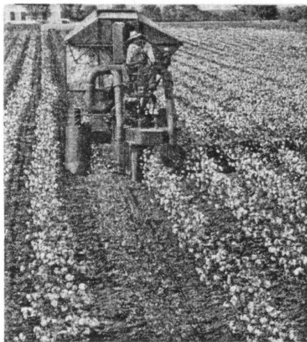
Fig. 1. Spindle picker operating under favorable conditions at Tennessee Valley Substation. Note clean-picked row, center.
