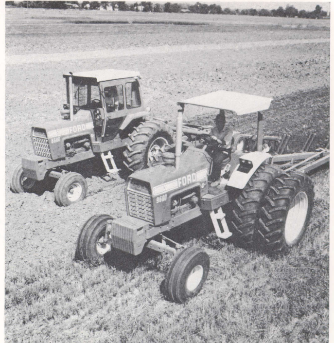
FIG. 2. Operator protection is available as standard equipment on most current tractors as a safety cab (left) or a protective frame (right) and can be purchased as separate items for mounting on older tractors.
