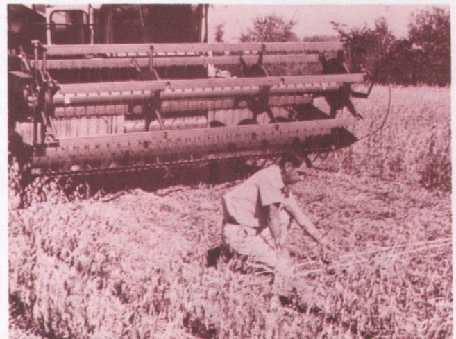
FIG. 2. Good combine operators frequently check for seed loss. Each four seeds per square foot represents 1 bu. loss.
