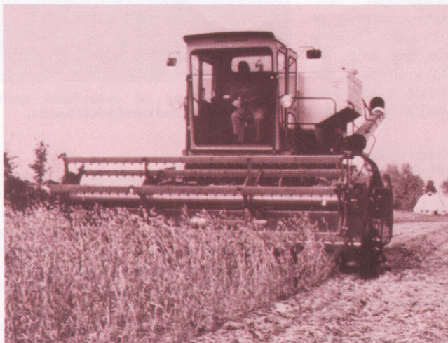
FIG. 1. Many soybean growers use a special pick-up reel on the combine to help reduce harvest losses.
