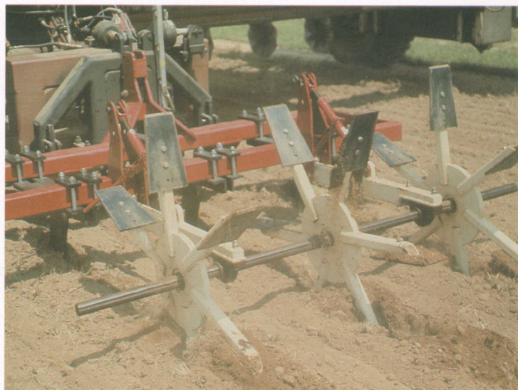
Water-holding reservoirs were made with this Dammer Diker.
