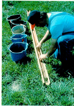
Soil cores were taken to bedrock.
