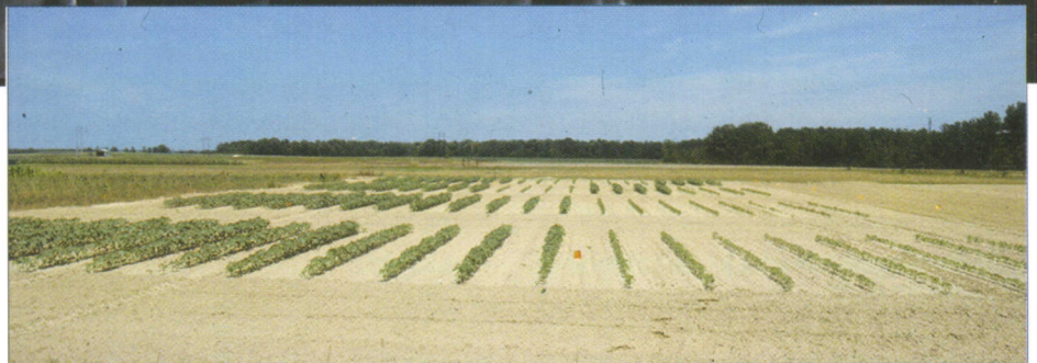
Sludge-treated plots (left foreground) had increased growth of seedling cotton and higher yields than conventionally fertilized plots (right foreground) in 1993.
