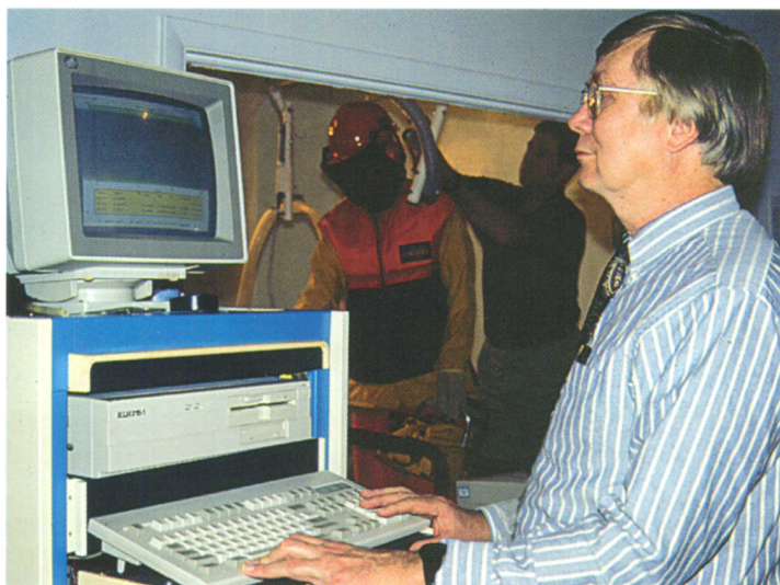
Auburn researchers use a multidisciplinary thermal laboratory to examine heat stress and other physiological responses to working in protective clothing, such as the garments worn by forestry wood workers.
