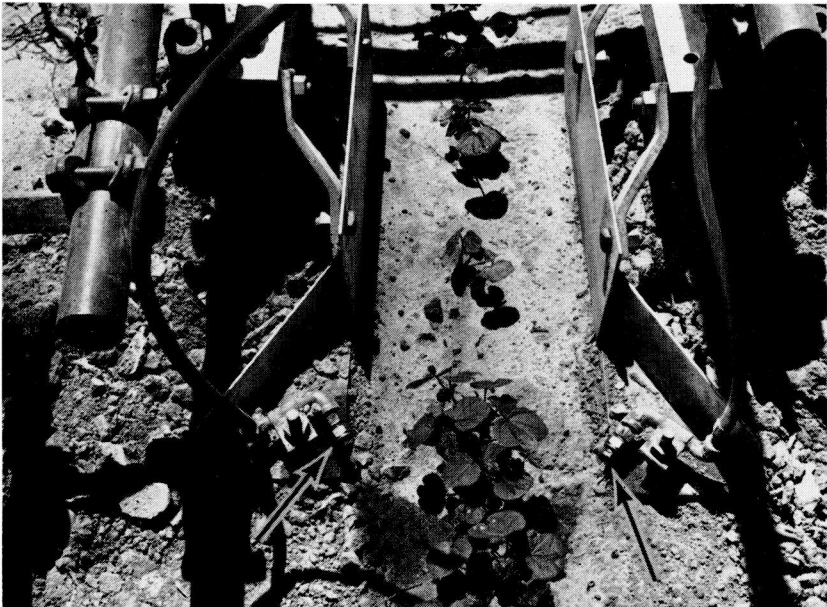
FIGURE 9. Shown are parallel action shields with nozzles (arrows) mounted for applying post-emergence chemicals. These shields prevent sweeps throwing dirt on the row when cultivating and applying post-emergence chemicals.
