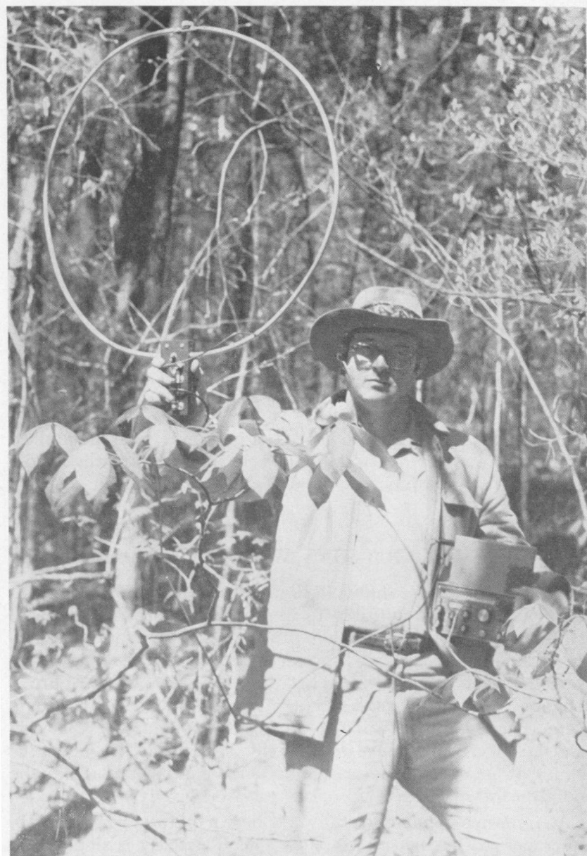
FIG. 4. Portable receiver and directional antenna used in monitoring raccoons in Lee Co., Alabama.
