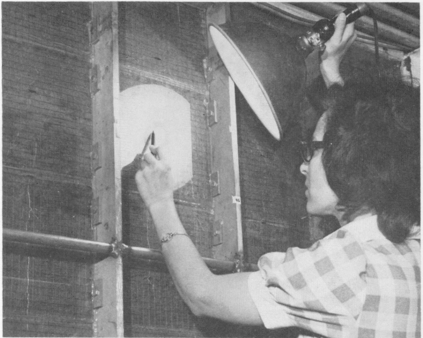
FIG. 3. Glass face of a compartment of the Auburn rhizotron showing the wire grid used as a reference for root measurements.
