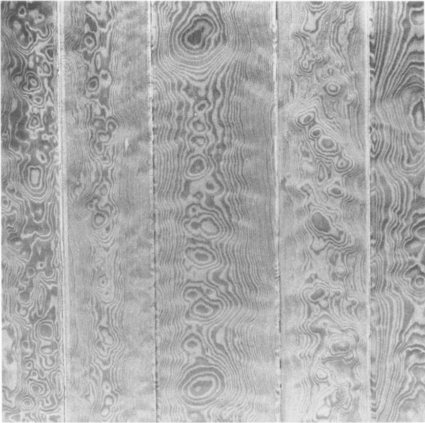
Figure 25. Wall paneling of curly southern yellow pine that shows typical blister figure characteristic of these woods (t).
