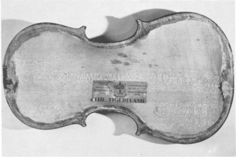
Figure 24. The inner-back surface of the instrument shown is Figure 23. Note the absence of fiddleback figure. Ray-fleck pattern is evident.
