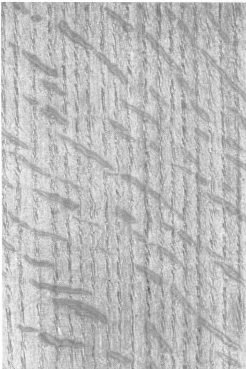
Figure 9. Typical ray-fleck figure in quarter-sawn oak (r).
