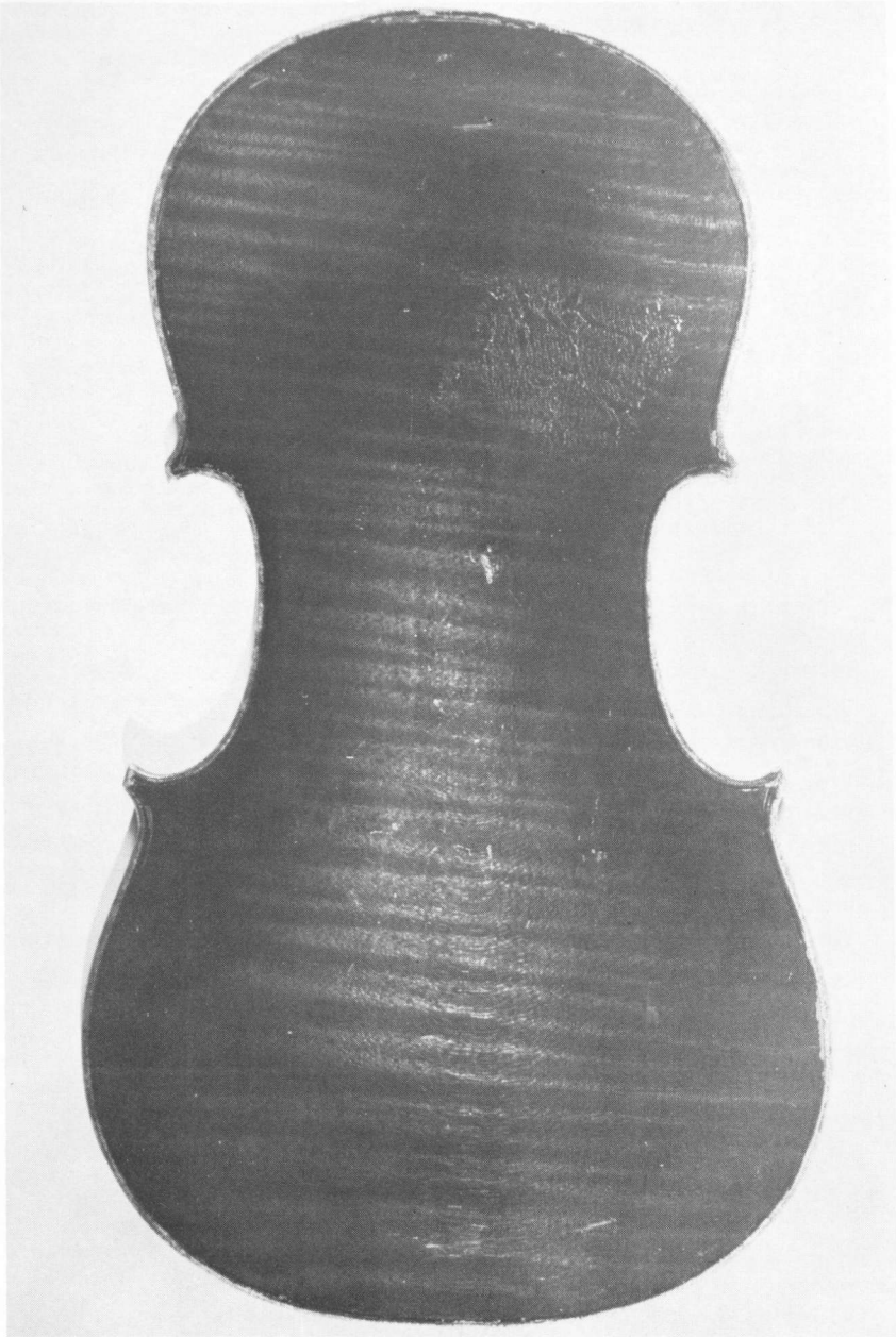
Figure 23. A violin back that illustrates a simulated fiddleback figure produced by staining (other types may be produced by acid etching or flaming).
