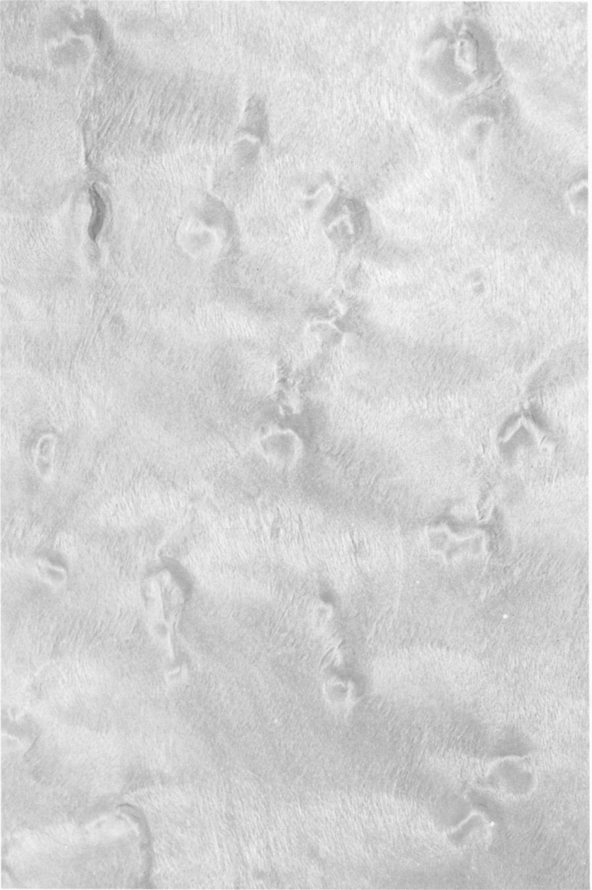
Figure 33. Birdseye figure of sugar maple in a veneer section (t) that illustrates typical figure pattern.
