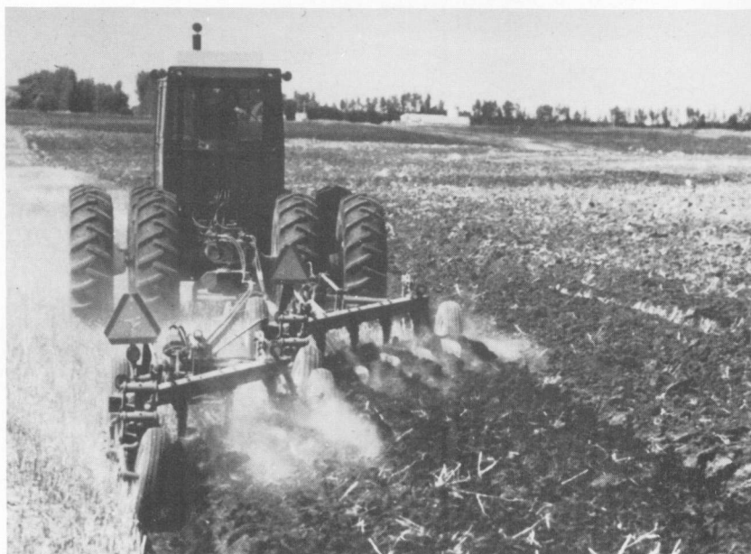
FIG. 12. Large fields and long rows are conducive to high field machine efficiency and increased machine capacity.
