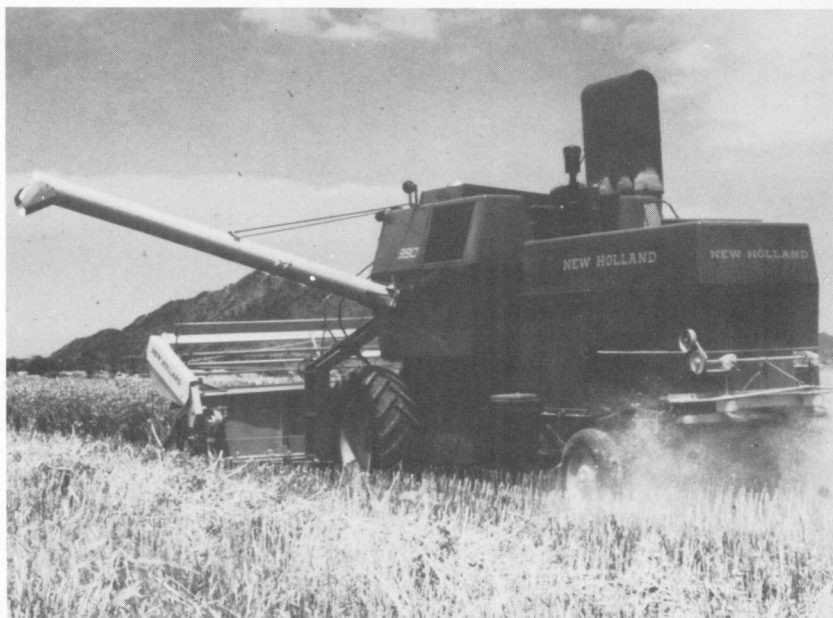
FIG. 11. Large self-propelled machines frequently need 20 to 30 feet of turning space.
