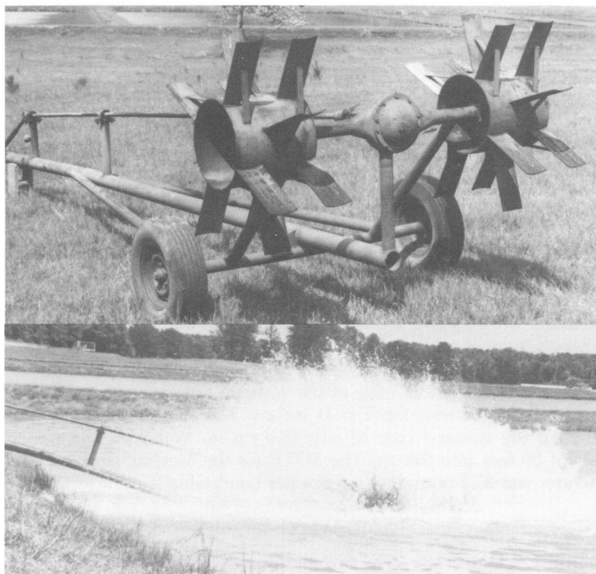
FIG. 8. Auburn University tractor-powered paddle wheel aerator.
