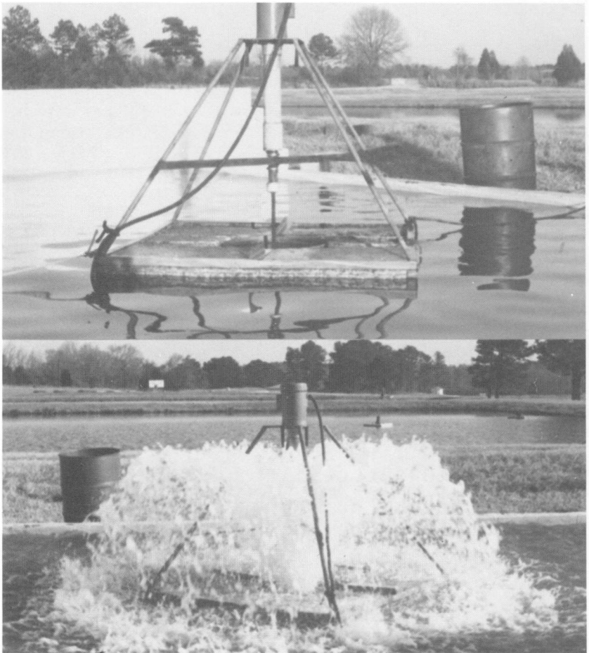
FIG. 26. Rogers vertical pump aerator.
