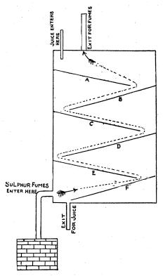
As indicated by the diagram, the shelves a, b, c, d, e, f, are arranged in a gently sloping position in order to permit of the easy, but not too rapid, flow of the juice through the apparatus, the sides and joints of the box being made as nearly air and water tight as possible, in order to provide against waste of either the juice or sulphur fumes.
