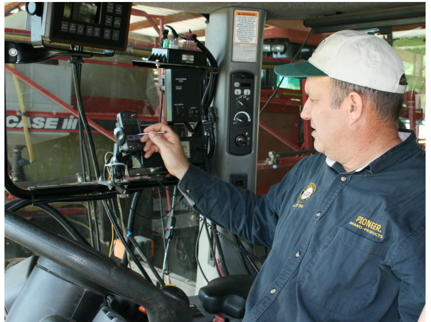
RIGHT ON THE MONEY —Don Glenn, who was one of the first farmers in the state to invest in precision ag equipment and systems, explains the navigational technologies that provide repeatable, centimeter-level accuracy for his field operations. Precision ag has helped Glenn reduce input costs, save time and labor and increase efficiency, productivity and profitability on his Glenn Acres farm in Hillsboro.
