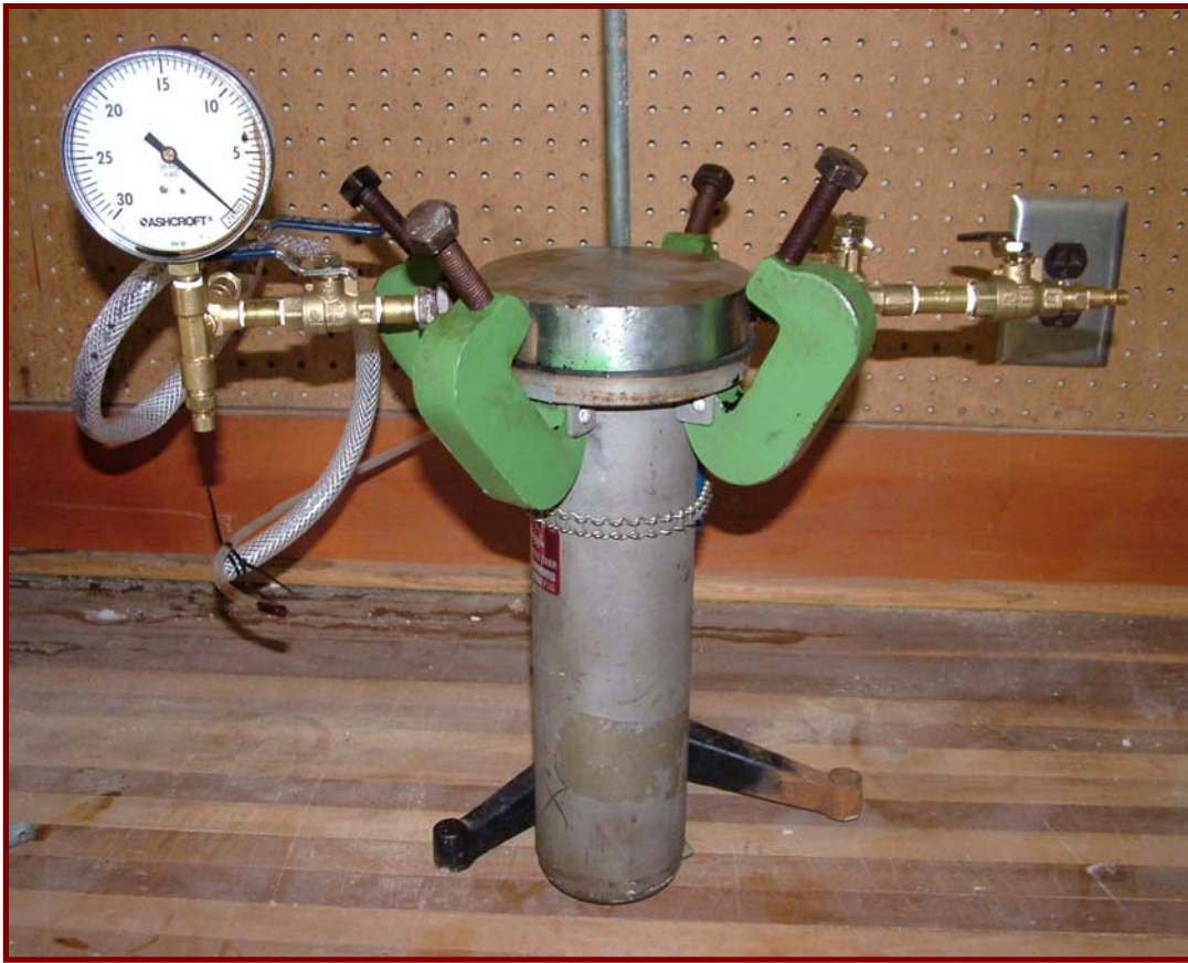
Fig. 1. Custom bench-scale vessel for high pressure treatment
