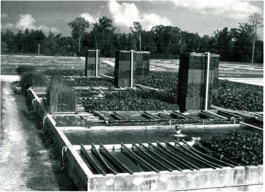
Figures 7a., 7b. A high intervention culture system. Although a biological filter and water circulation were used, there was no effort to control water temperature. This system, used to culture tilapia, was not operated during the winter.
