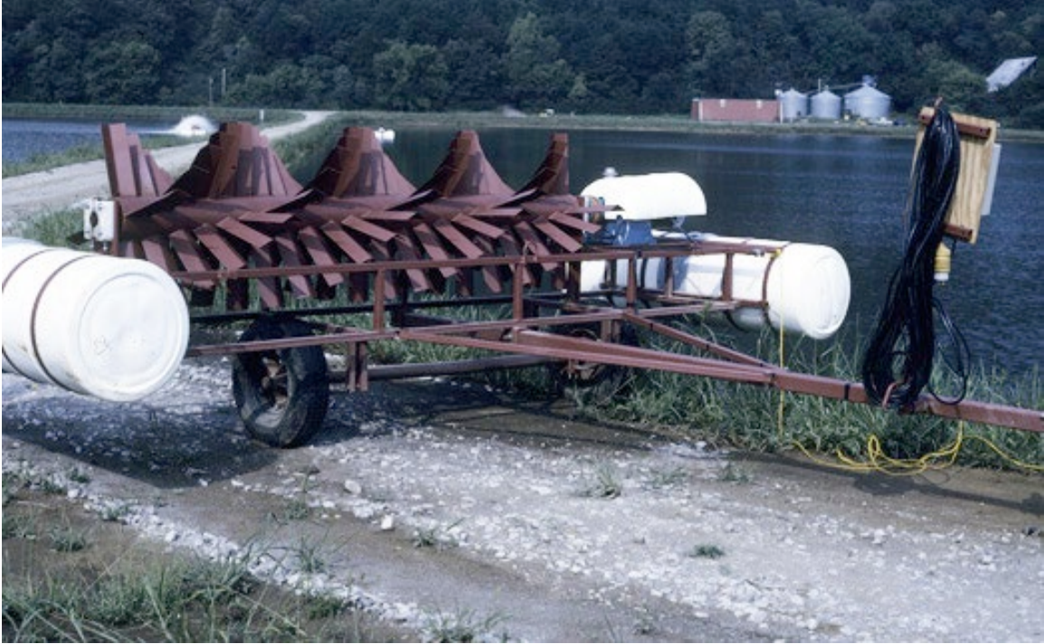
.Figure 105. Pond aeration device designed by Boyd and his Work Group.
