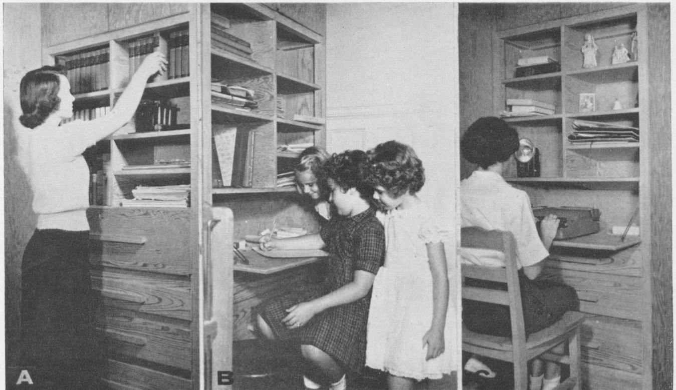
FIGURE 26. Original desk unit in use: (A) books when removed from shelf were caught by frame above; (B) children
