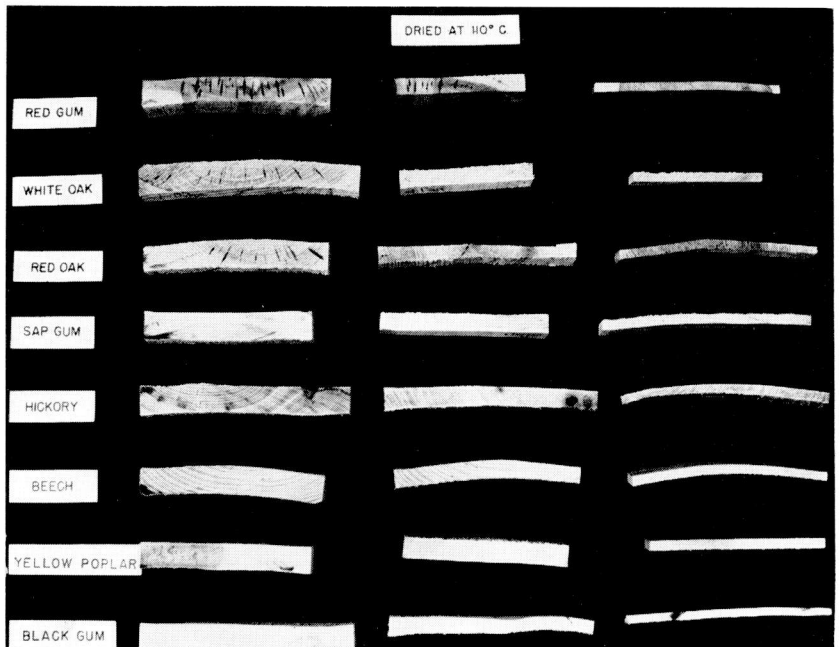
Figure 2. Cross sections of boards of various species that were dried at 110° C. The sections on the left are from \frac{3}{4} inch, in the center from \frac{1}{2} inch, and on the right from \frac{1}{4} inch boards.
