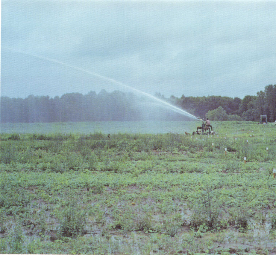
Water collected at various points under irrigation provide data used by the computer to design application patterns to give more uniform application of water by hose-towed traveler and towable pivot irrigators.
