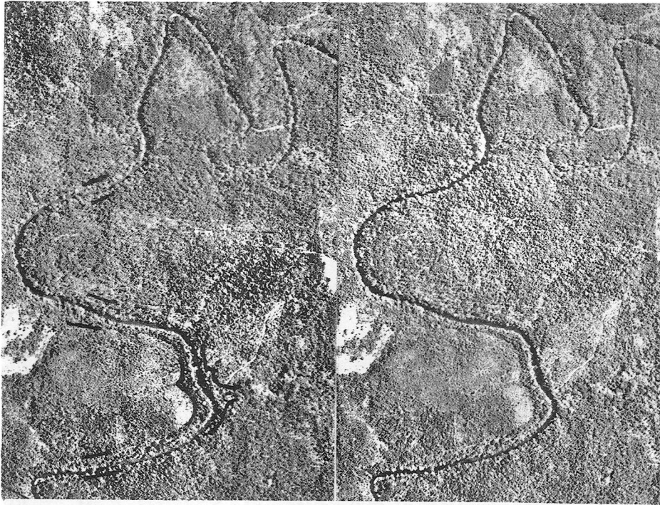
FIGURE 15. Stereogram of a stream that is somewhat wider than 30 feet (Tallapoosa County). The extent of the floodplain is marked at several points. (APC-1JJ-212,213)
