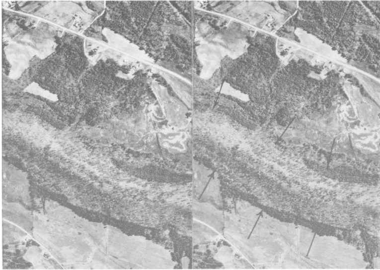
Figure 6. Stereogram showing a northeasterly-striking linear ridge of Fort Payne chert in Zone I. Surrounding the ridge is the relatively flat terrain of Zone IX. Note the sharp boundary between the two zones. In addition, note the symmetry of the cross-section of the ridge, which is typical of chert ridges. (Calhoun County, GR-2LL-165, 166).
