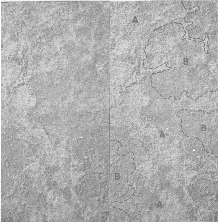
Figure 18. Stereogram showing a portion of the "flatwoods" in Zone IV. The slight relief on this area is clearly evident. In the area labelled (A) the relief is so gentle that slope positions cannot be assigned. Consequently such areas have been classed as "flat." In the area labelled (B), relief is slight but hills can be distinguished. These should be recognized as such when using the key. (Cherokee County, GT-2LL-221, 222).
