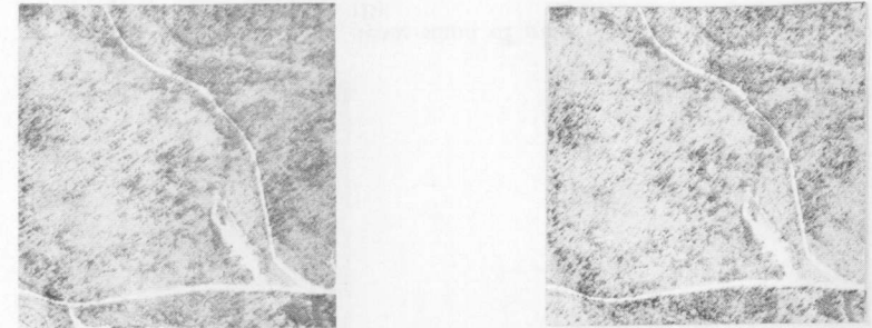
Figure 41. Stereogram of a medium-stocked, mixed pine-hardwood stand. The photographs were taken in the spring before leaf development was complete. The hardwood component is revealed primarily by shadows.
